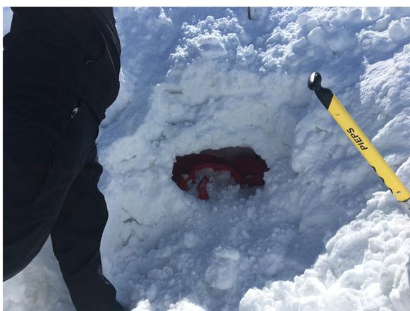
**Fig. 3 – Example of the air pocket created by deflation of the airbag observed upon extrication.**
