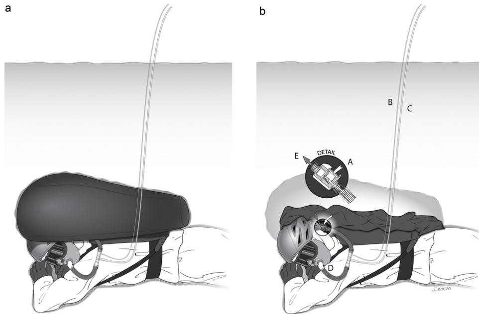
**Fig. 1 – Experimental setup. (a)** Depicts conditions after inflation of the airbag at time 15 s–3 min after trigger. **(b)** Depicts conditions after deflation of the airbag at 3 min.
