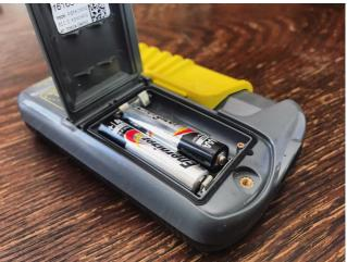
4. Check for corrosion on the batteries and in the battery compartment. If there's corrosion in the battery compartment, then clean it off with a Q-tip and rubbing alcohol—especially the battery contacts. Remember, corroded battery contacts are not warranted by any beacon manufacturer as they are considered user error.
